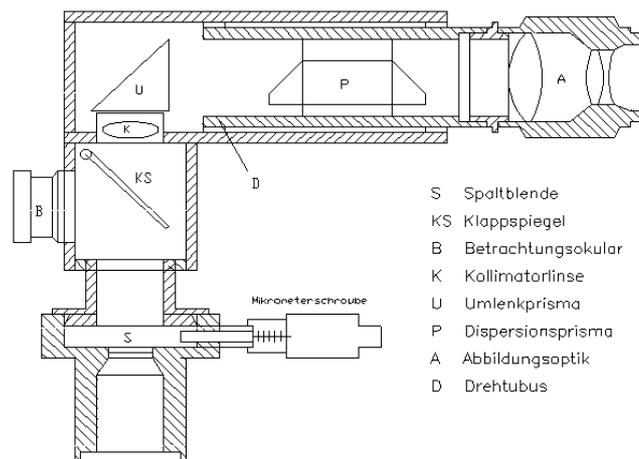
**Figure 1:** S Slit, KS Flip mirror, B control ocular, K collimator lens, P dispersion prism, A imaging lens (ordinary photo lens).
