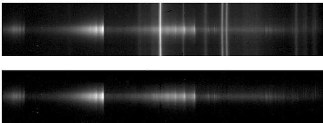
**Figure 4:** Raw CCD spectra of comet Ikeya-Zhang on 2002-Apr-22 in the range approx. 470 nm – 630 nm. Top: with background (the 546.1/577.0/579.1 nm Mercury lines are visible). Bottom: background subtracted.
