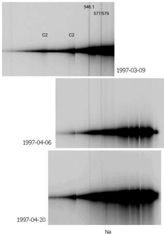
**Figure 3:** This composite image shows three raw CCD images. On April 20, the Na emission is visible. The image taken on Apr 06 shows also a very weak emission on the same position (probable not visible here in the paper; see [2] ).
