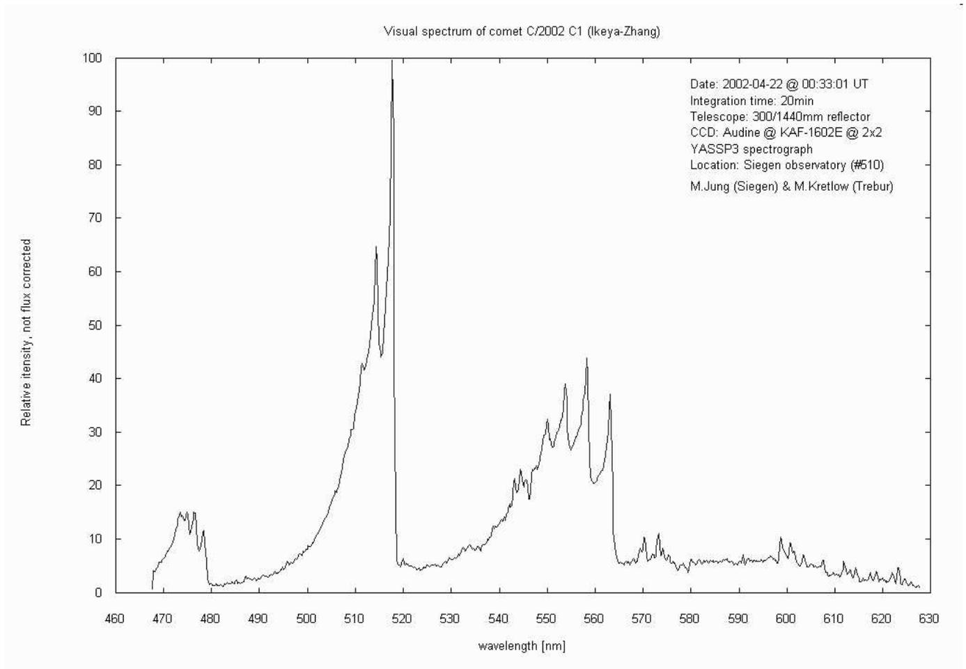
**Figure 5:** Preliminary reduced spectrum of comet C/2002 C1 (Ikeya-Zhang), taken on 2002-Apr-22 with the YASSP3 spectrograph on a 300/1440mm Newton reflector. The slit was centered on the head of the comet. The intensity is scaled to 100% for the strongest emission ( $C_2$  at 515nm). Some of the smaller peaks between 570nm and 630nm should belong to  $NH_2$  and probable to  $H_2O^+$ , but apparently no sodium emission is detectable.
